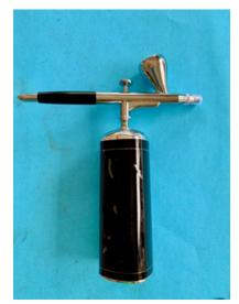
It is a hand held air compressor with a detachable air brush. I originally purchased just the compressor and figured I would attach an Iwata or Badger airbrush to the top. Unfortunately, a Badger or Iwata will not mate with the compressor.
