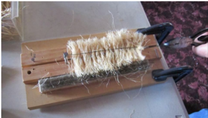
The second clinic was mainly about making twisted fiber conifers using this homemade device to secure and twist fibers cut from sisal. Presented by Dick Roberts, MMR
