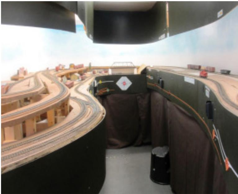
*Above:* This shot shows how Ben has added schematic diagrams, color-coded turnout controls, and other visual aids for operators, to the valance and fascia.
